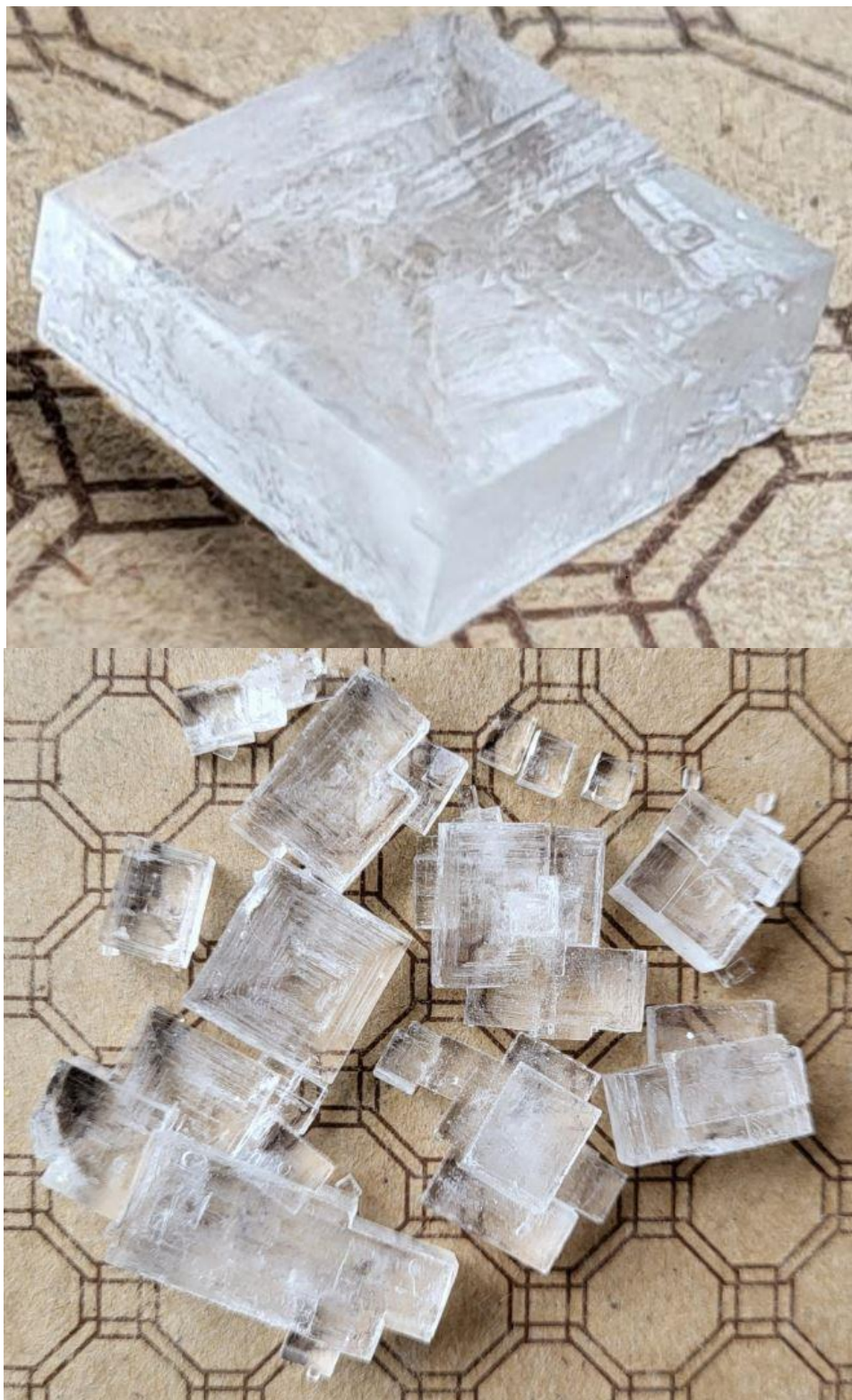
Figure 1 KCl crystals grown from slow evaporation of a saturated potassium chloride solution.
