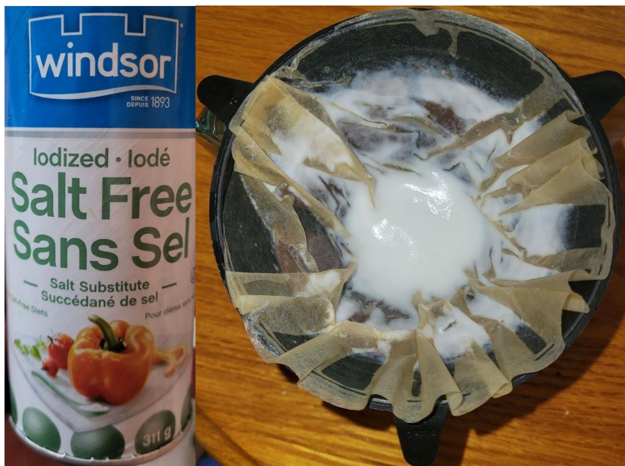
Figure 2. Example of a grocery store available source of potassium chloride (left) and the insoluble anti-caking agents which can be removed via filtering hot solutions of the salt. Evaporation then gives potassium chloride crystals, which can be recovered from solution, or the solution can be dried thoroughly to afford purer potassium chloride. Ensure the ingredients contain no sodium chloride, and only potassium chloride (commonly alongside things like sugar, potassium iodide, magnesium carbonate, and calcium silicate).
