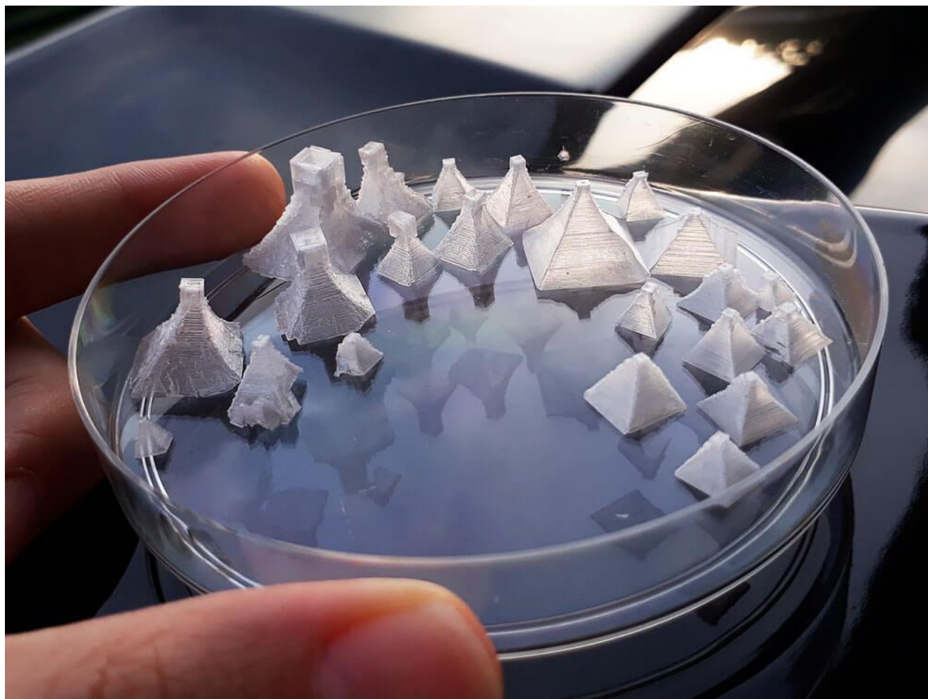
Figure 3. Example of some of the incredible tutorials available at crystalverse by Chase Lean. These crystals of sodium chloride (table salt, NaCl) are grown following a specific procedure which allows for isolation of these pyramid structured crystals.
