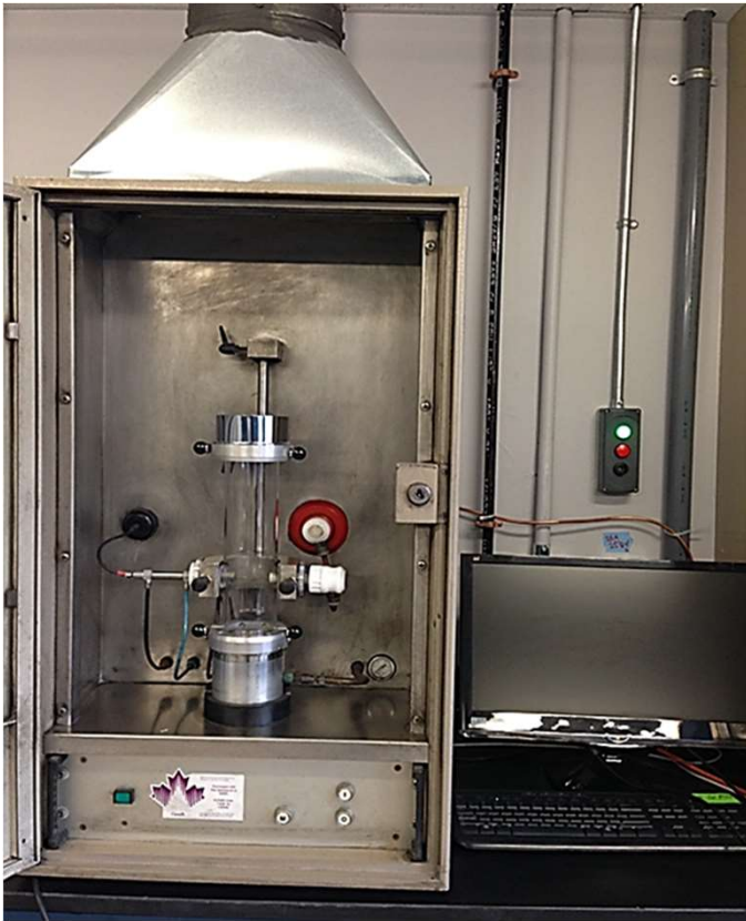
MIKE-3 apparatus – testing per ASTM E2019-03 (2013)
