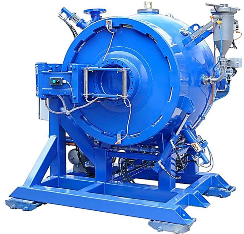
OZM 1-m 3 chamber at Fauske – testing per ASTM E1226-13 (2018); E1515-14 (2018)
