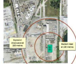
Figure 15: Proposed HTEC Fatality Risk Contours for Radiant Heat and Explosion Shockwave Impacts
