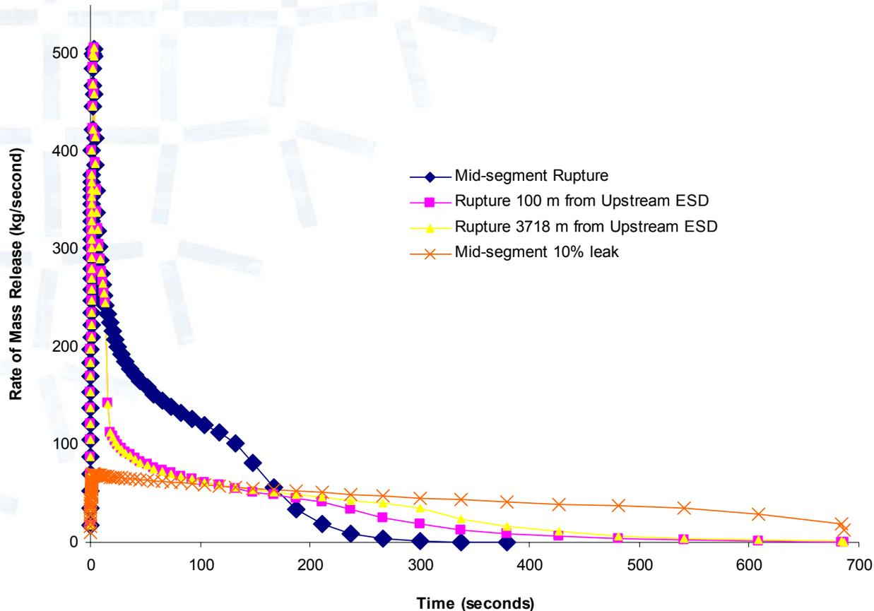
When the rates of mass released during upstream, downstream and mid-segment ruptures are compared with a mid-segment 10% leak scenario, it is apparent that the leak scenario could result in a higher TWA exposure to the public.
